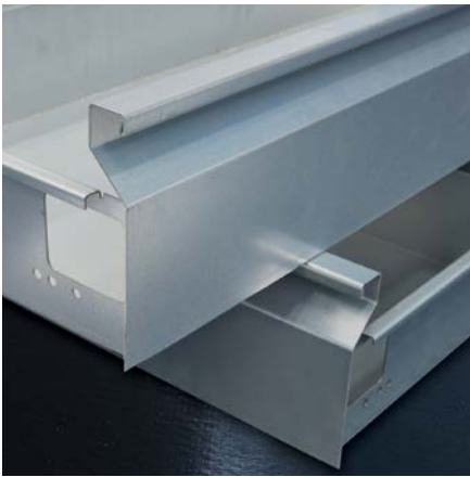
Sheet metal parts produced with PSBB manufacturing line for metal furniture industry.
